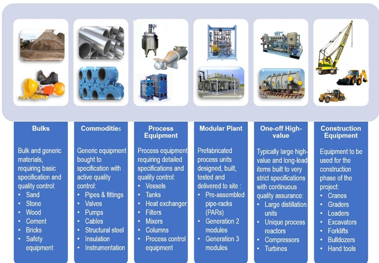
**Figure 3: Materials, components and equipment for a process plant**
