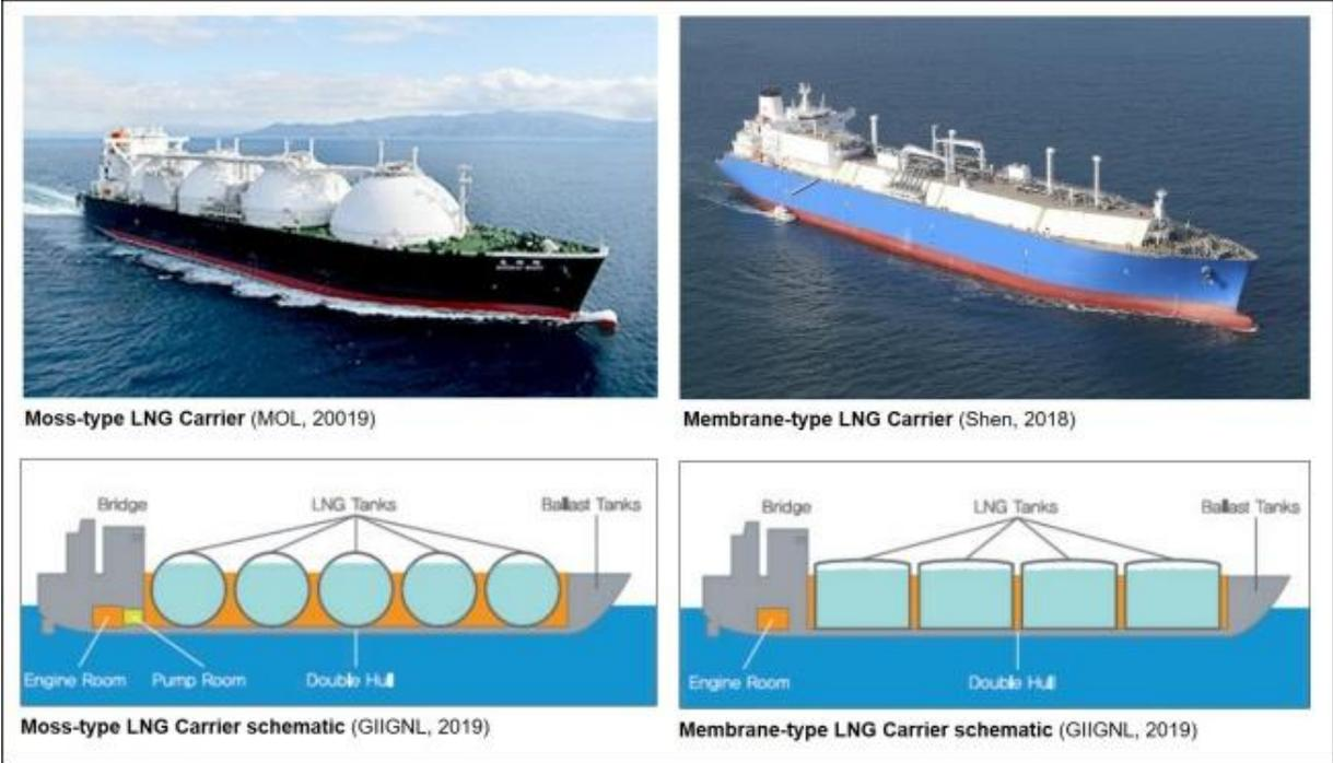
**Figure 7: Moss-type and membrane-type LNG carrier vessels**
