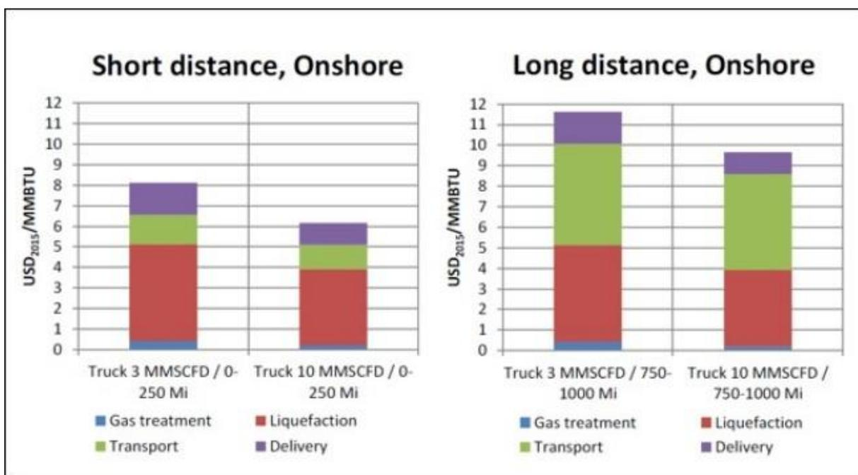
Figure 11: Comparison of LNG onshore transport costs (Tractebel Engineering, 2015)
