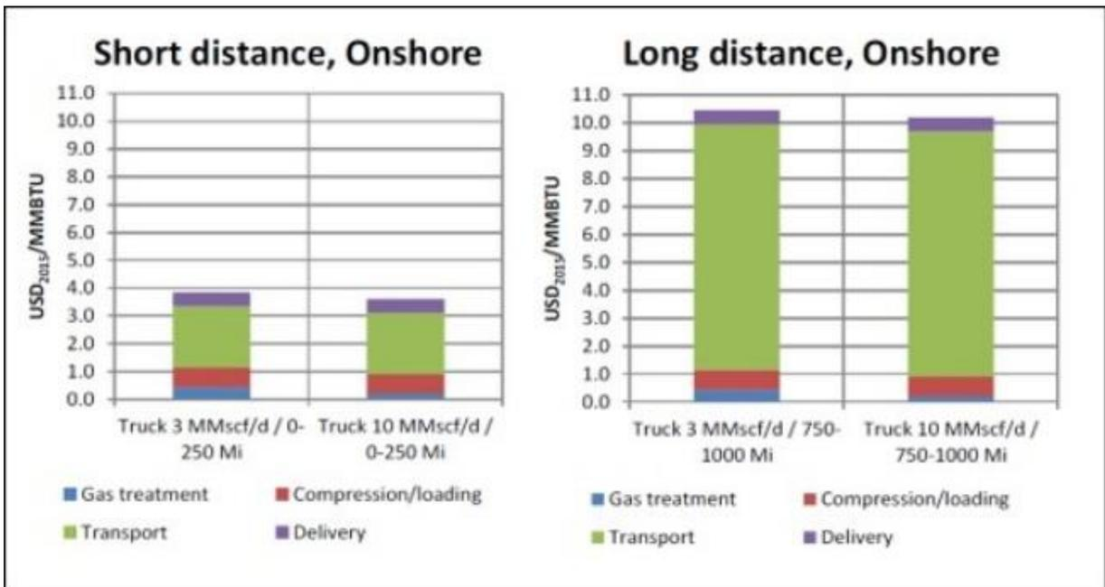
**Figure 5: Comparison of CNG onshore transport costs** (Tractebel Engineering, 2015)
