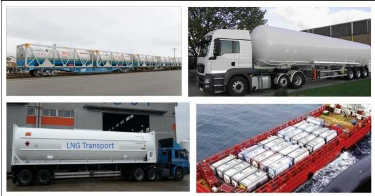
**Figure 10: Transport options for LNG with tankers and ISO containers**
