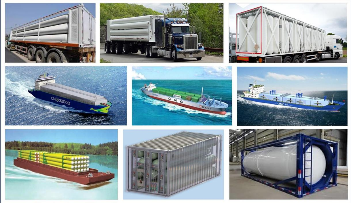
**Figure 4: Different options for transporting CNG**
