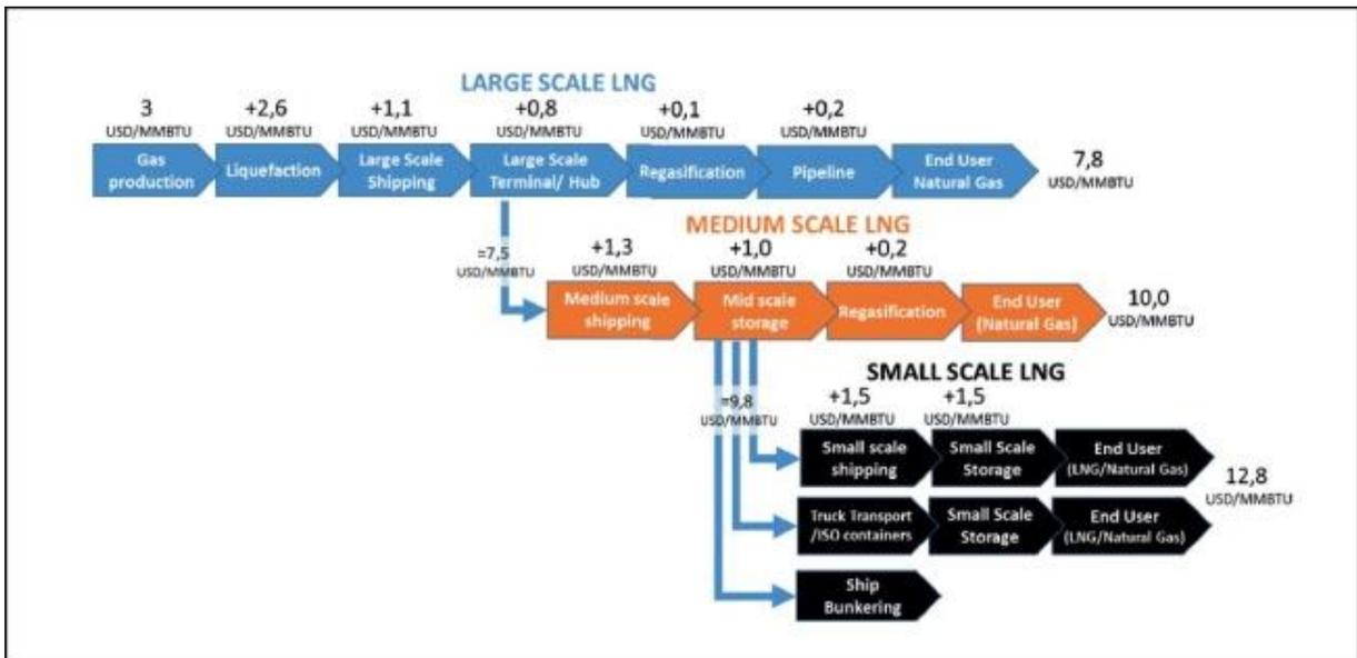
Figure 8: Offshore marine LNG logistics chain example (Wärtsilä, 2017)
