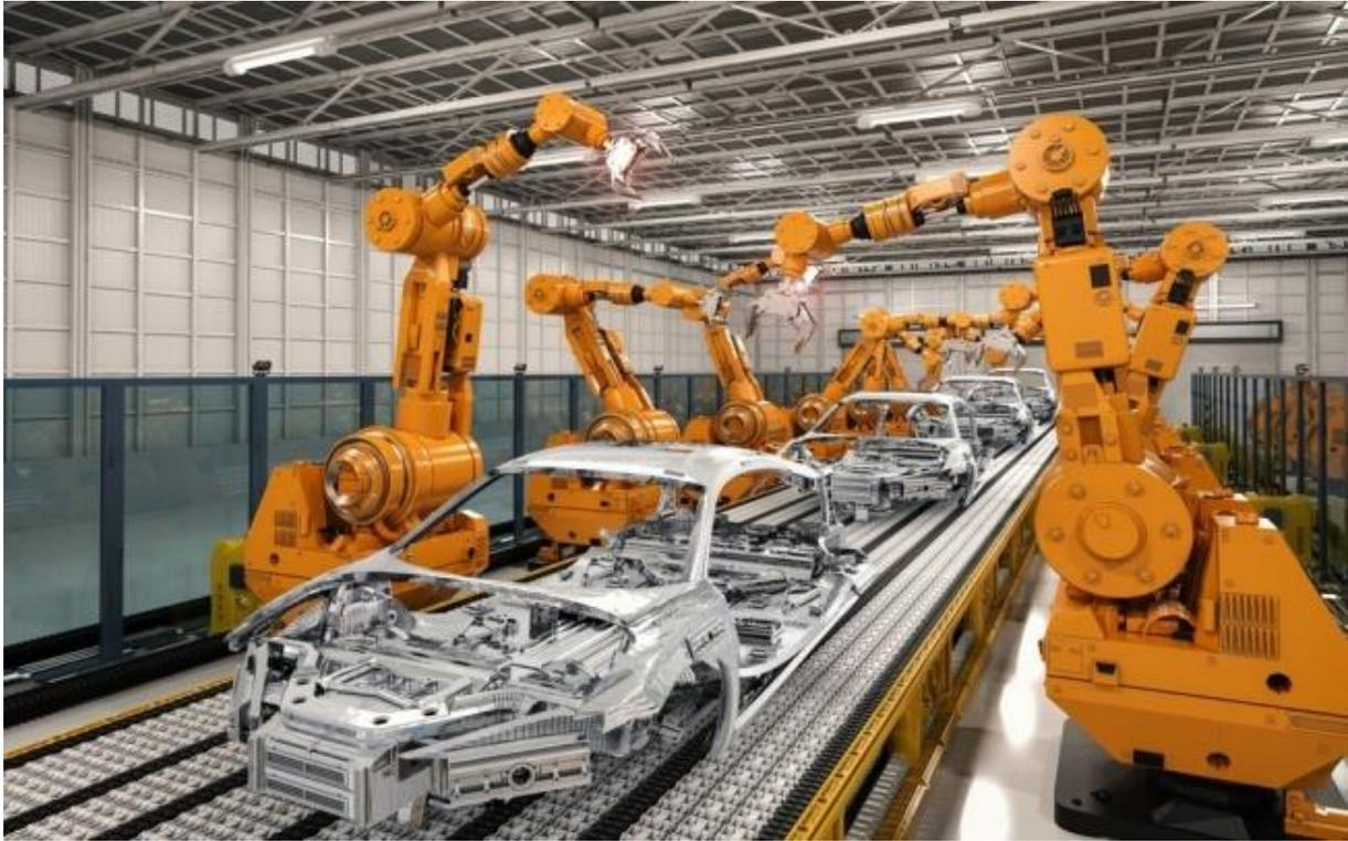
**Figure 3: Automated robots used in a vehicle assembly application**
