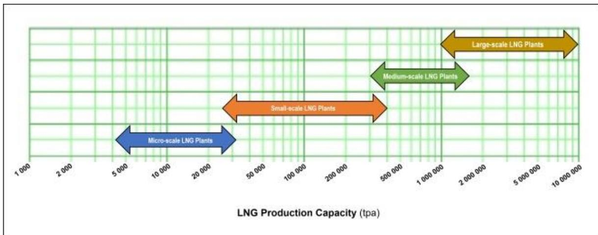
**Figure 1: Terminology for liquefaction plant size**
