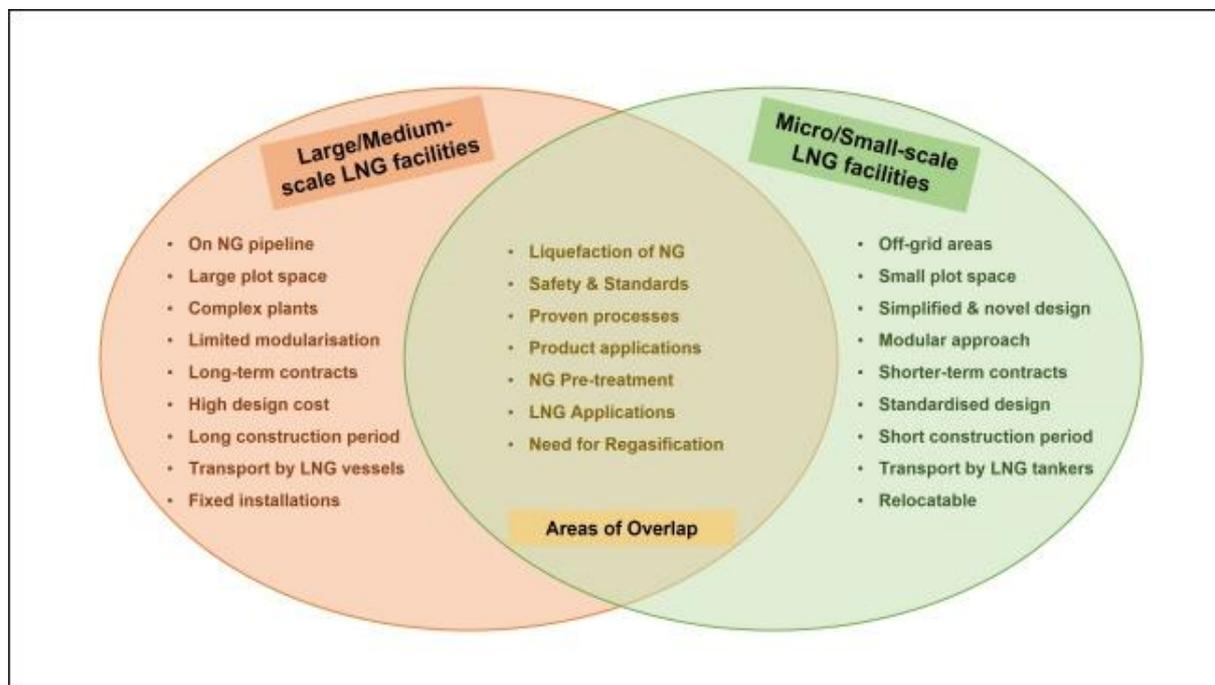
**Figure 3: Comparison of small-scale LNG and large-scale LNG**
