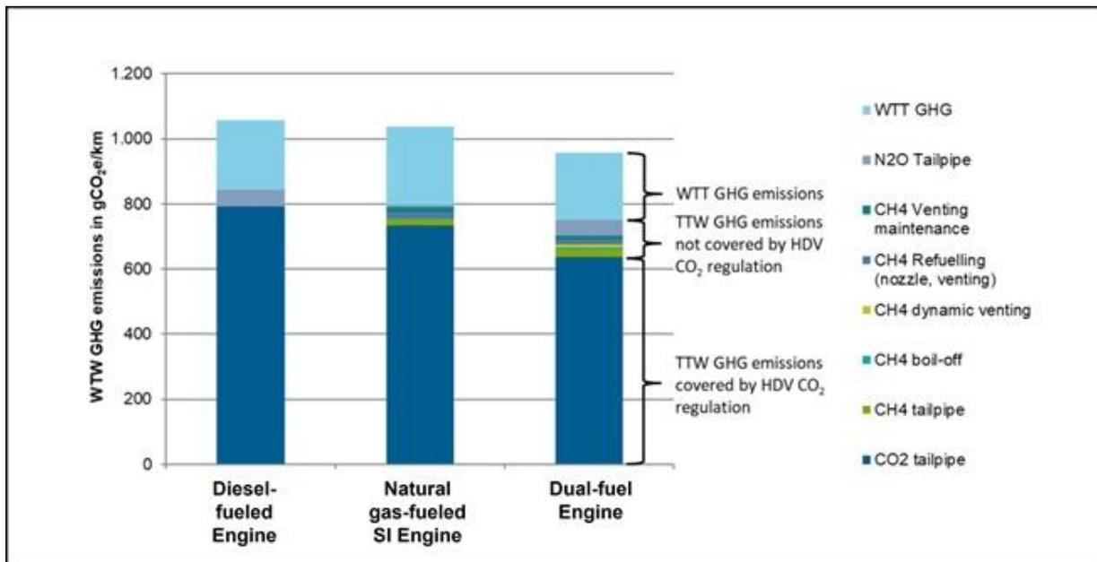
**Figure 7: GHG emissions for various engines** (adapted from Mottschall et al, 2020)
