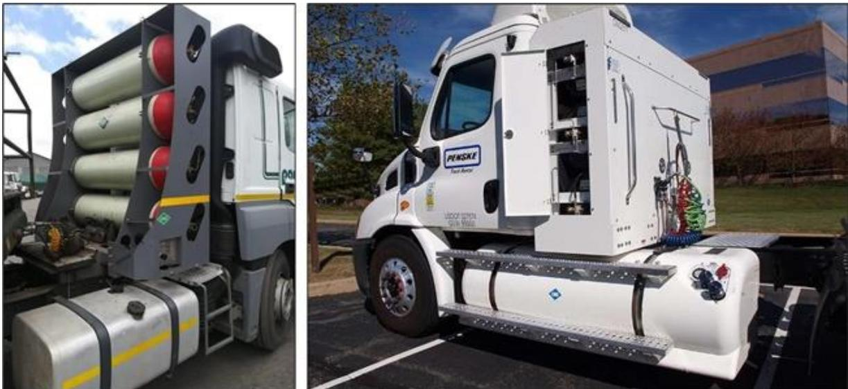
**Figure 2: Back-of-cab and frame-mounted CNG fuel cylinders**
