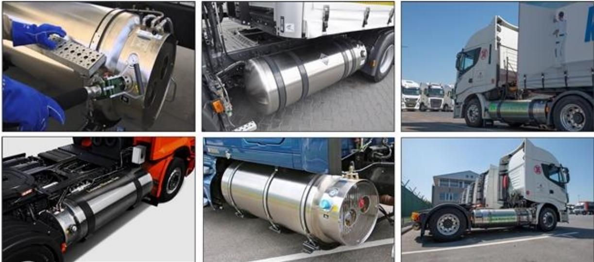
**Figure 3: LNG tanks on heavy duty trucks**
