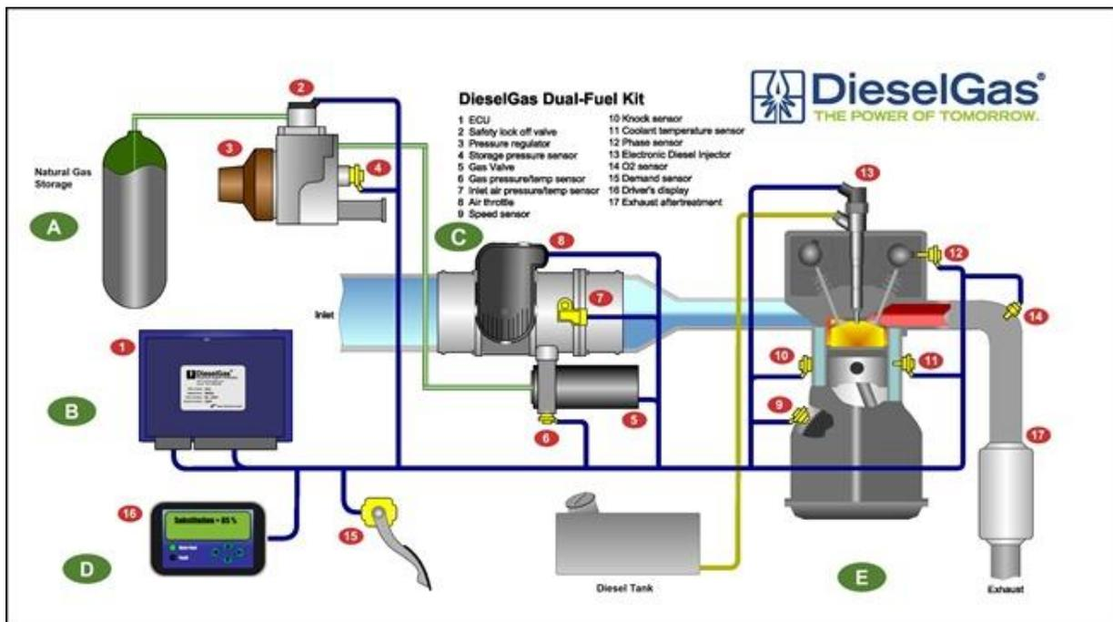
**Figure 6: Schematic of a dual-fuel system (DieselGas, 2021)**
